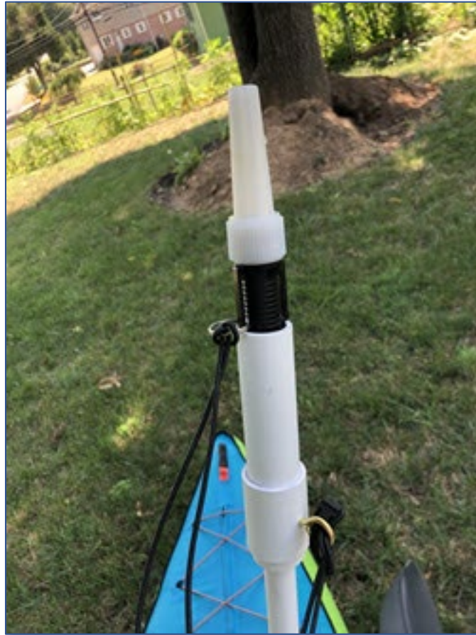
Figure 7 - Closeup of Light Socket with Light
