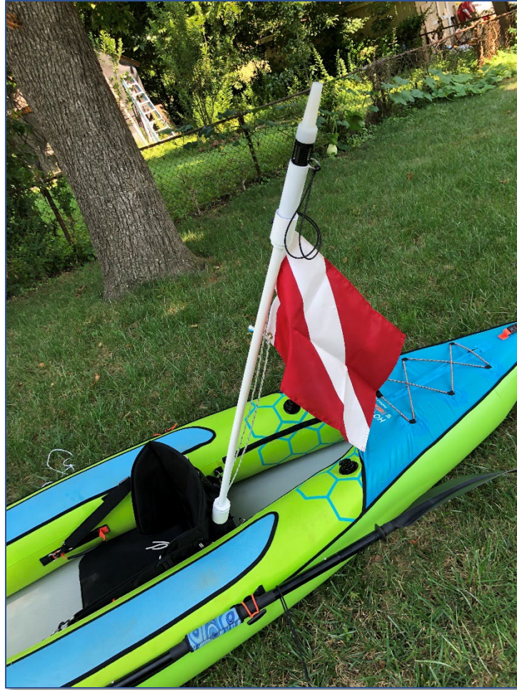
Figure 2 - Mast Rigged with Light and Dive Flag
