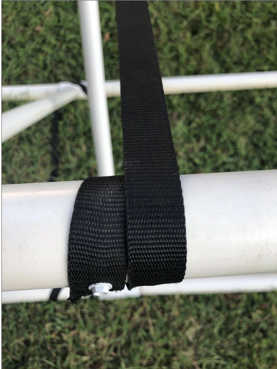
Figure 13 - Detail of Nylon Strap Installation
