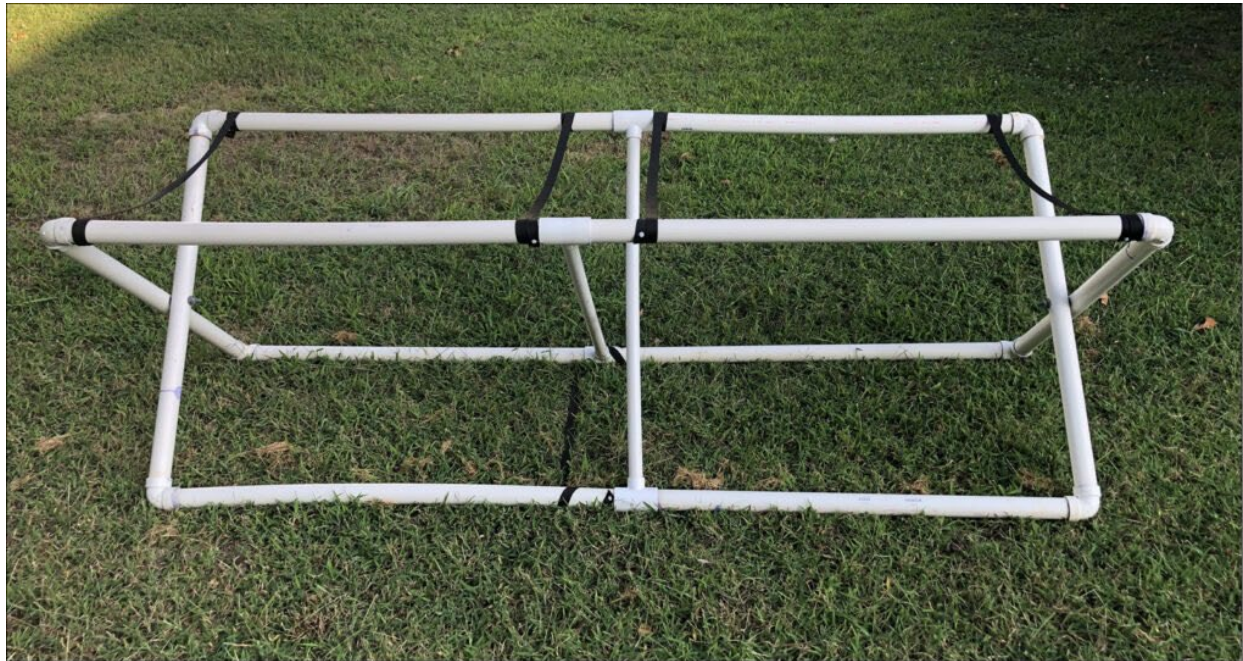
Figure 1 - Kayak Work Stand Built of PVC Piping and Nylon Straps
