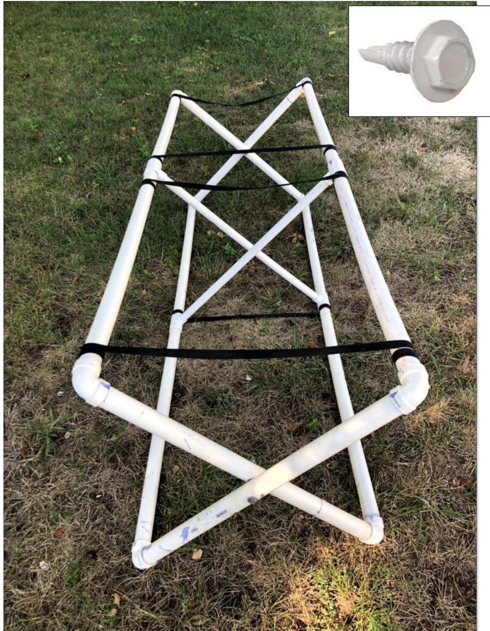
Figure 4 - View Showing the Nylon Straps and Detail of Self-Drilling Screws
