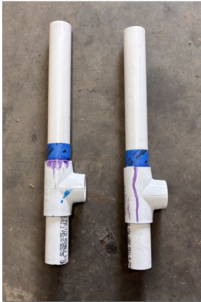
Illustration 6: Use Painters Tape to Mark Alignment
