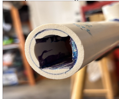
Illustration 10: Showing the Squared Inner Section of the PVC Axle
