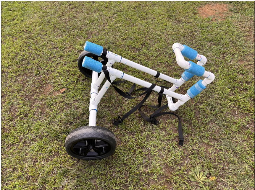
Illustration 1: Home built Cart for the Native Watercraft Slayer Max 10
