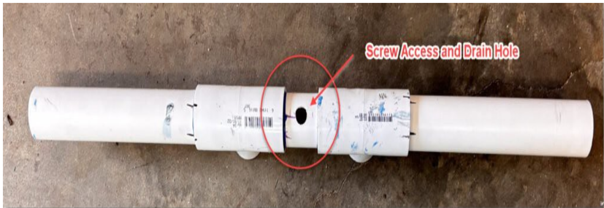
Illustration 11: Detail Showing Access Hole for the Axle Screw, and A Drain Hole
