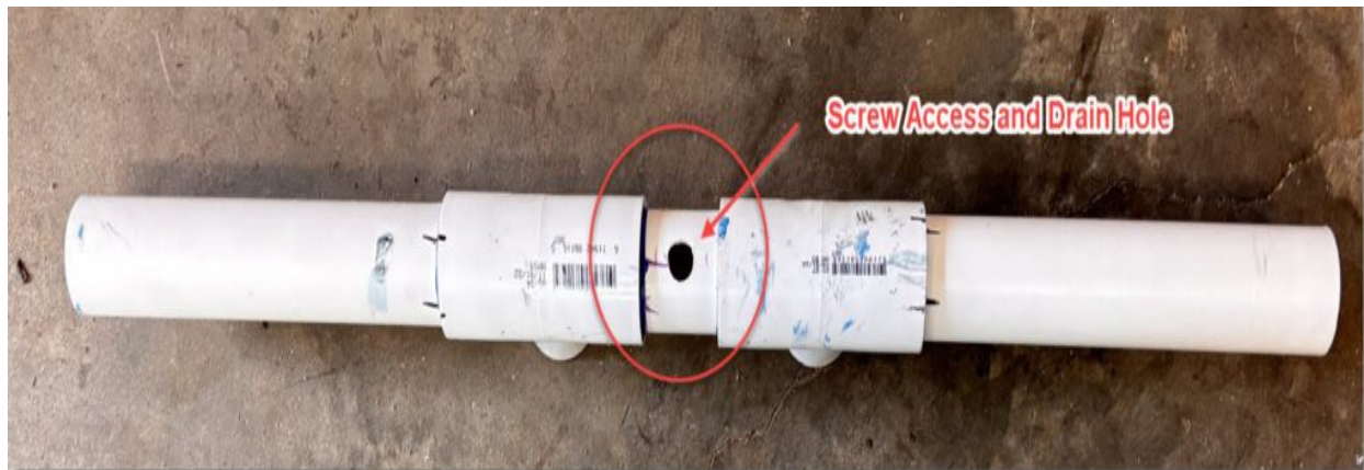
Illustration 12: Detail Showing Access Hole for the Axle Screw, and A Drain Hole
